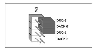
Figure 2-9. DMA Jumper Setting for No DMA Channel
